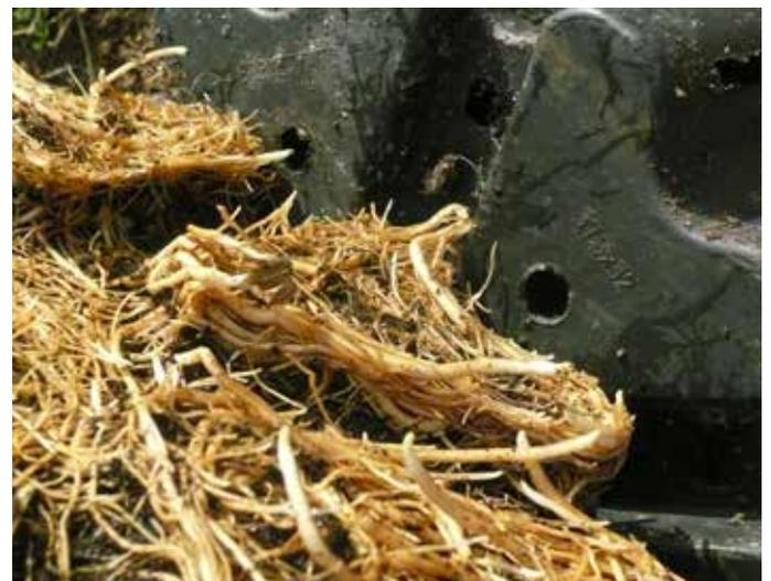
The **growth and the expansion of the roots as well**, are the main reasons of the deterioration and loss of elasticity: this is why **Ercole** and **Varia** have some introflections that break such expanding forces keeping the structure.
