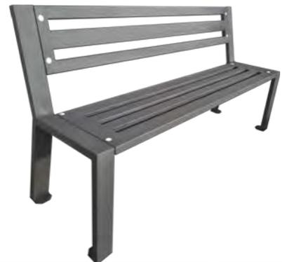
Bruxelles style bench, consisting of 2 tubular galvanized iron supporting sides with rectangular section, provided with socles at the base, pre-set for being laid on the ground and/or for the securing with anchors bolts, length 1750 mm, width 530 mm, height 830 mm. Seat (dim. 390x1750 mm) and back rest (dim. 400x1750 mm) constituted by panels made by galvanized iron tubular slats, secured by means of steel bolts.
